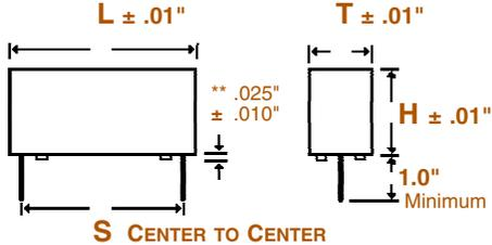
\*\* The mounting pads consist of two individual pads on each end or one continuous pad on each end, depending on the mold. (Not an option).
